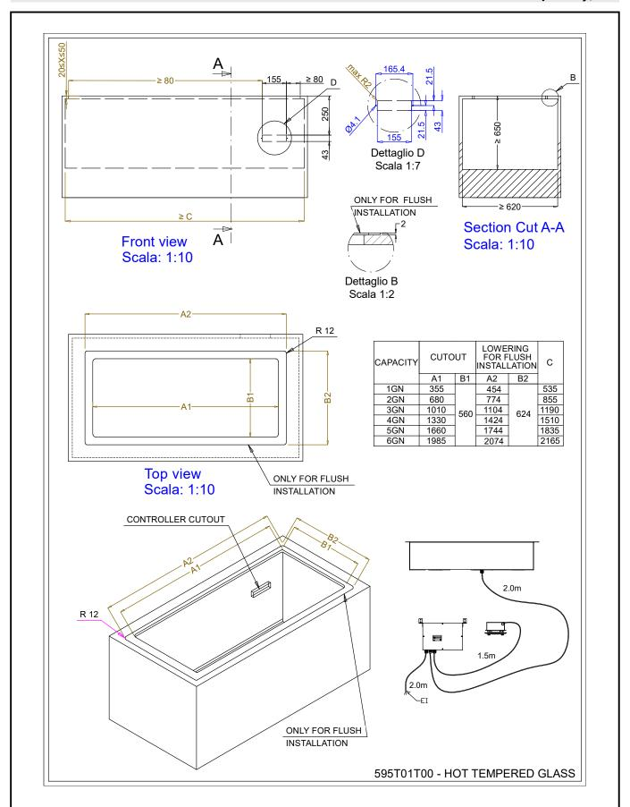
Drop-in tempered glass top (2 GN container capacity)
